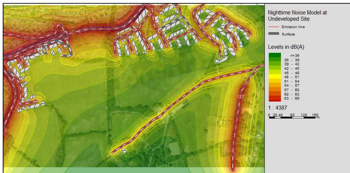
Figure 10.7 Noise Model of Nighttime LAeq at the Undeveloped Site
