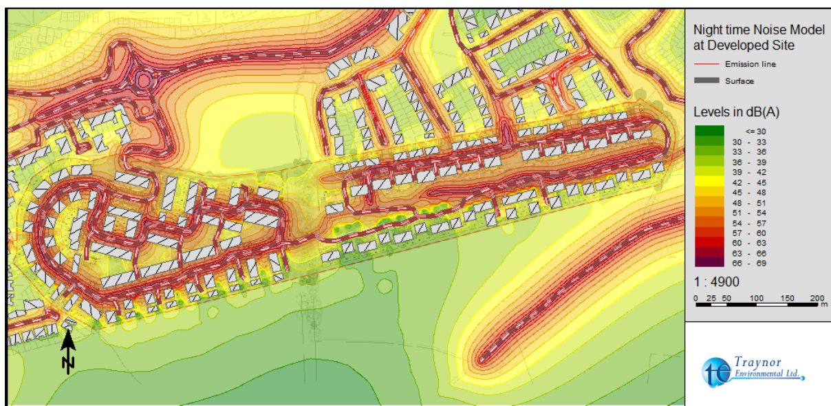
Figure 10.9 Noise Model of Nighttime LAeq at the Developed Site
