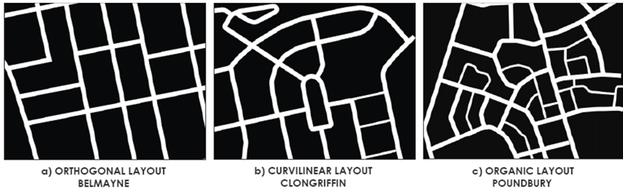
Figure 6 | Permeable Street layouts (Source: Figure 3.8 – DMURS)
