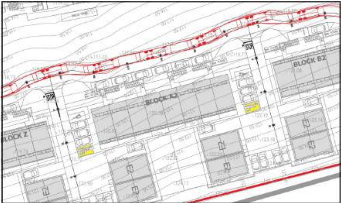
Figure 19 – Refuse truck Autotrack and servicing of bin areas
