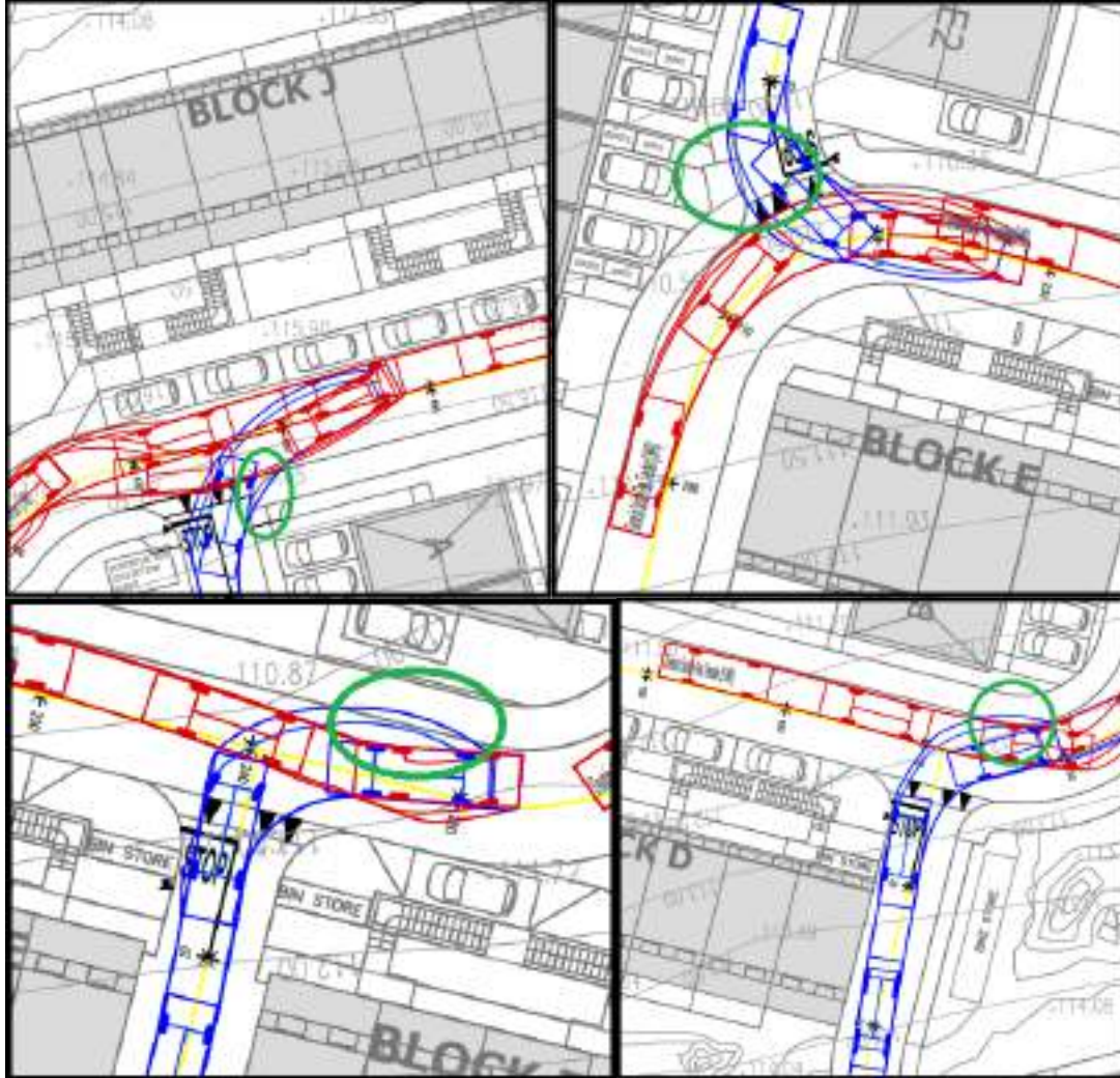
Figure 20 – Fire Tender Autotrack issue
